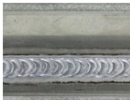
Fillet weld, 8 mm sheet metal, AlMg, argon 1.2 mm wire electrode Perfect ripples, thanks to superPuls
