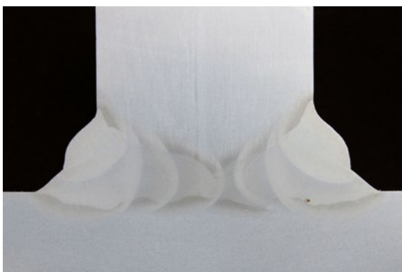
S355, t = 30 mm, double bevel seam with 35° included angle, welded without air gap on both sides, without gouging or grinding on the root concavity side
